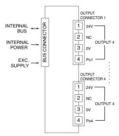
Note: Pin 1 of output connector is connected to 24V of the excitation supply. Pin 1 of output connector is connected to 0V of the excitation supply.
