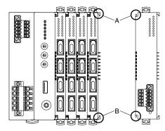
Confirm that the locking clamps of the extension power supply module are set. Insert the module in parallel to the next one while aligning the grooves of both modules (A & B in the above figure). Maintain it perpendicularly to the rail.
