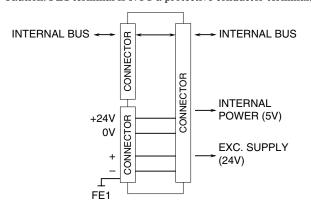
Internal bus is connected for the modules near to the power / network module out of the modules connected to the R8-PS1. Internal power and Exc. supply are not connected. All modules far from the power / network module are connected.
