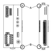
Confirm that the locking clamps of the I/O module are set. Insert the module in parallel to the next one while aligning the grooves of both modules (A & B in the above figure). Maintain it perpendicularly to the rail.
