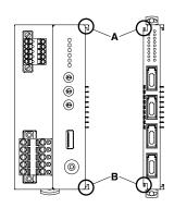
Confirm that the locking clamps of the I/O module are set. Insert the module in parallel to the next one while aligning the grooves of both modules (A & B in the above figure).
