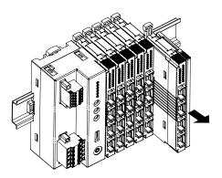
Removing an intermediate module
