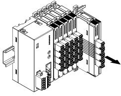
• Removing an intermediate module
