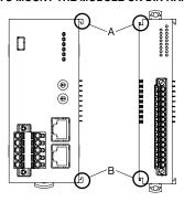
Confirm that the locking clamps of the extension power supply module are set. Insert the module in parallel to the next one while aligning the grooves of both modules (A & B in the above figure). Maintain it perpendicularly to the rail.
