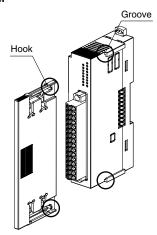
The protective cover is to be attached over the connected I/O module at the right end.
