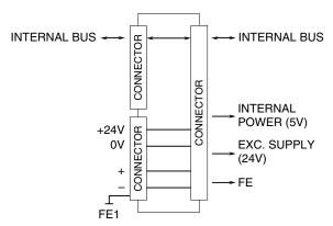
Internal bus is connected for the modules near to the power/ network module out of the modules connected to the R80PS1. Internal power and Exc. supply are not connected. All modules far from the power/network module are connected.
