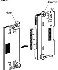
The protective cover is to be attached over the connected I/O module at the right end.
