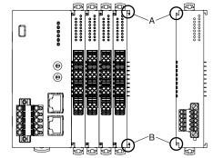
Confirm that the locking clamps of the extension power supply module are set. Insert the module in parallel to the next one while aligning the grooves of both modules (A & B in the above figure). Maintain it perpendicularly to the rail.
