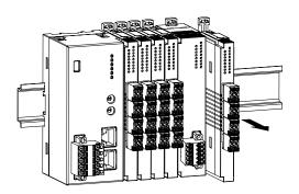
Removing an intermediate module
