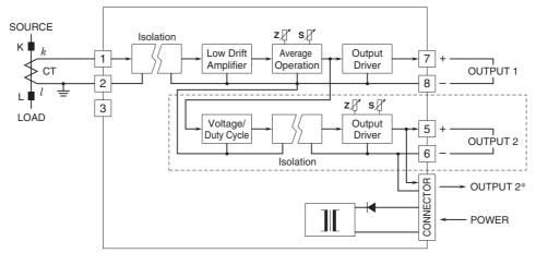
\*1 output type has the output 1 connected to the card-edge connector in parallel. Remark 1) The section enclosed by broken line is only for 2nd output channel.
