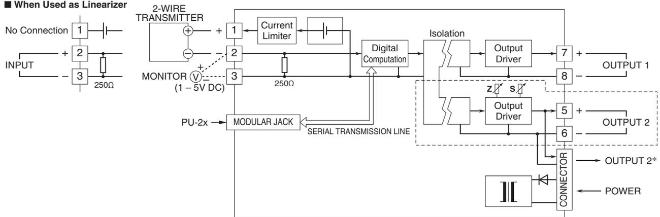
\*1 output type has the output 1 connected to the card-edge connector in parallel.
