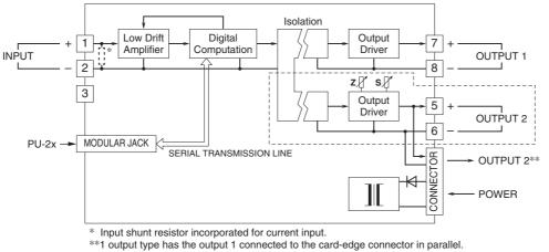
Remark 1) The section enclosed by broken line is only for 2nd output channel.
