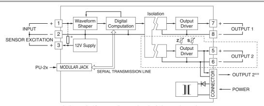
\*  $4k\Omega$  attached for open collector and mechanical contact input only. \*\*1 output type has the output 1 connected to the card-edge connector in parallel. Remark 1) The section enclosed by broken line is only for 2nd output channel.
