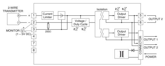
For OUTPUT 2 with current output, use eihter of terminals on the front or connector on the rear.
