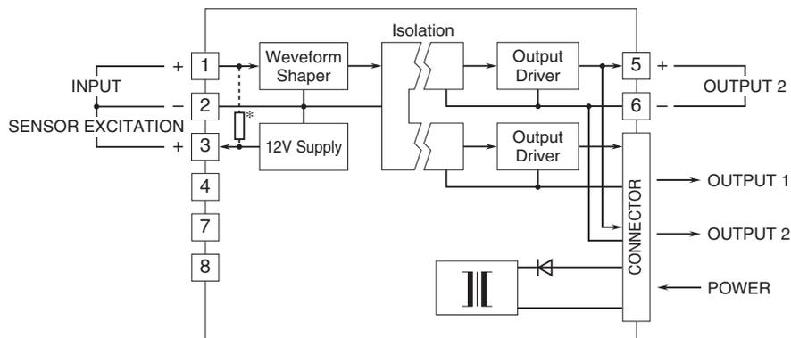
\*4kΩ attached for mechanical contact and open collector input.
