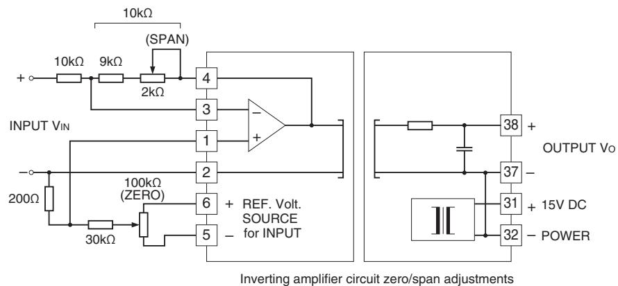
Inverting amplifier circuit zero/span adjustments
