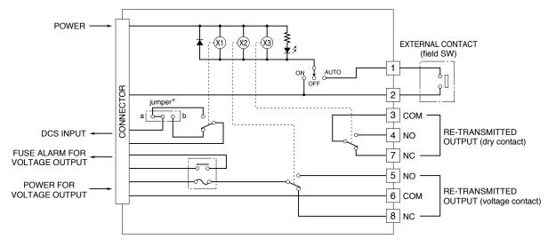
\*The jumper is factory set N.O. (position "a") Select position "b" for N.C.
