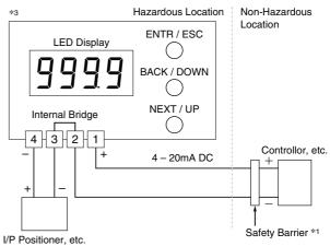
$<sup>\</sup>ensuremath{^{*}\text{1.}}$  A safety barrier must be installed for the intrinsic safety.
