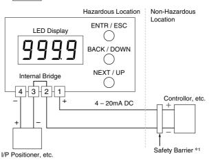
The safety barrier must meet the Ex-data of this unit and must be approved for the hazardous location.
