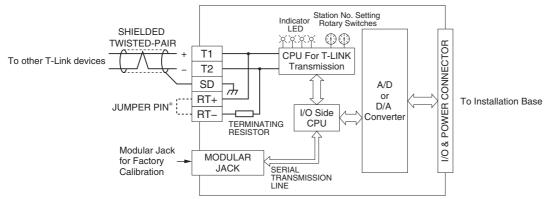
\* When the unit is located at the end of transmission line via twisted-pair cable (= no cross-wiring), short across terminals RT+, RT- with the jumper pin (or wire) provided with the unit.
