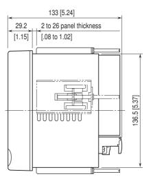
Attach the mounting bracket either on the top/bottom or on the sides.
