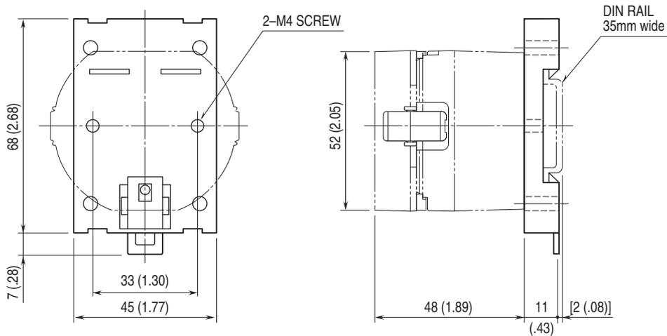
Leave enough space at both sides of the module to reach the side levers when installing/removing the LCD module.
