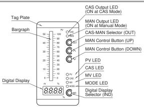
• Type 5: 5.5  $\leq$  Scale Span < 11.0 Number of divisions: 22 to 43.9 Scale: Starts at 0, increments in 0.01 / 0.1 / 1 / 10 / 100 / 1000. Min. and max. values are indi-cated. 4 digits including negative sign and decimal point. **Division lines**: Long, Medium, Medium, Medium, Long (5 divisions repeating)
