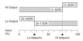
Trip Operation in Power Failure
