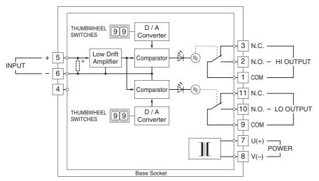
$* Input \ shunt \ resistor \ incorporated \ for \ current \ input.$
