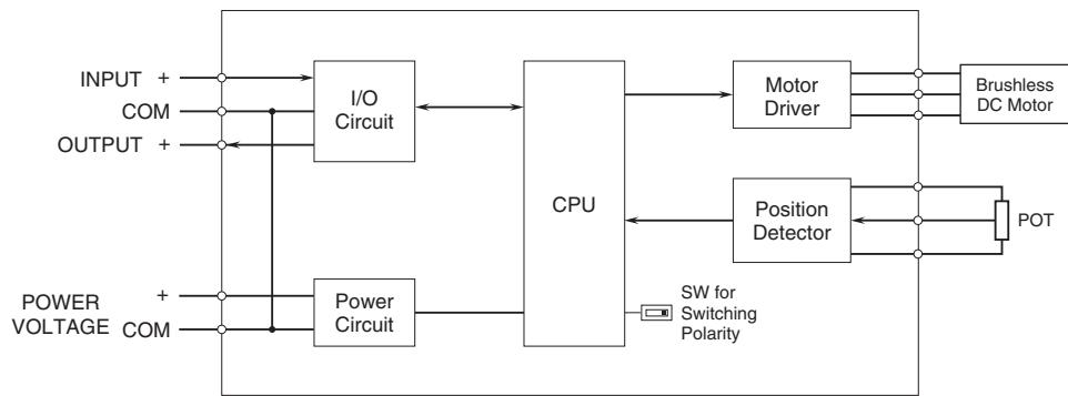
The COM port of the power is connected to the COM port of the input/output. Ensure proper alignment when connecting AC power.
