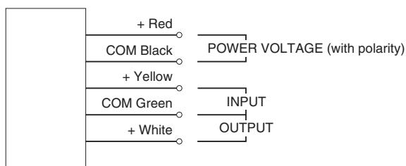
The COM port of the power is connected to the COM port of the input/output. Ensure proper alignment when connecting AC power.
