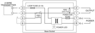
\*The DS-48 incorporates a resistor [ $100\Omega \pm 5\%$ ] for adijusting load on the current loop (\*\*). When the resistor is not required, short across terminals 5-6, or connect the 2-wire transmitter to terminals 3(+)-6(-).
