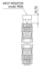
Input shunt resistor attached for current input.
