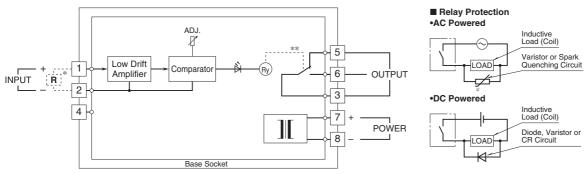
\* Input shunt resistor attached for current input. \*\*Relay status is determined by output codes.
