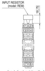
Input shunt resistor attached for current input.
