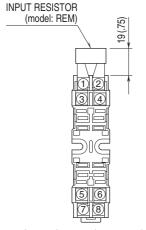
Input shunt resistor attached for current input.
