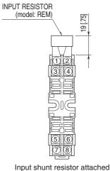
Input shunt resistor attached for current input.
