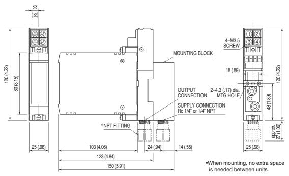
\*Fitting is provided for 1/4" NPT connection.
