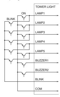
Note: If "On" and "Blink" are set simultaneously for a single lamp, "Blink" is disabled.
