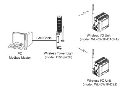
■ Modbus Master (PC side) communicates with Slave Devices in multi drop connection on the wired side (RS-485) via wireless connection using Modbus/TCP and RTU protocols.
