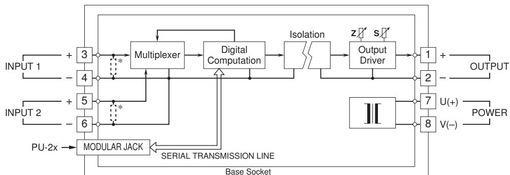
\*Input shunt resistor incorporated for current inputs.
