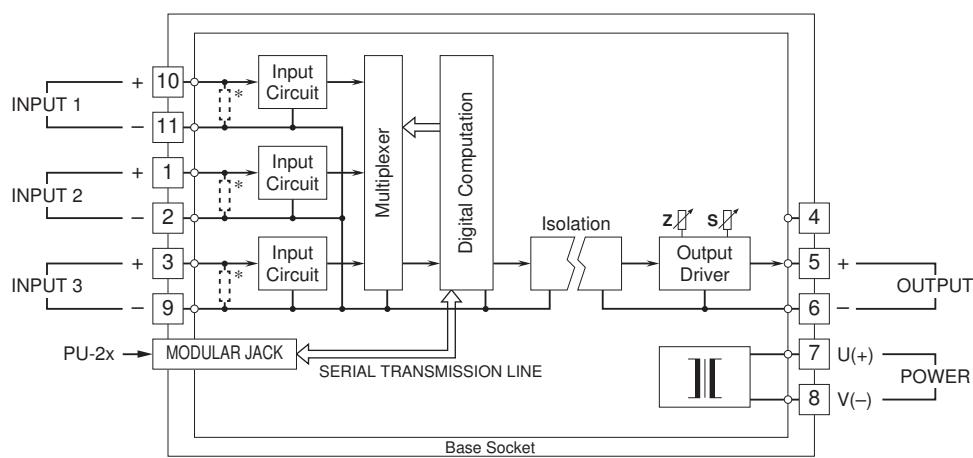
\*Input shunt resistor incorporated for current inputs.
