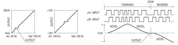
Forward Rotation: Phase A leads the Phase B by 90 degrees. Reverse Rotation: Phase A lags behind Phase B by 90 degrees.
