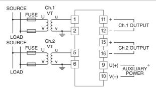
\*The transducer can be powered from the input voltage when the voltage is sufficiently stable and meets within the range of auxiliary power supply of the unit specified in the data sheet/instruction manual.
