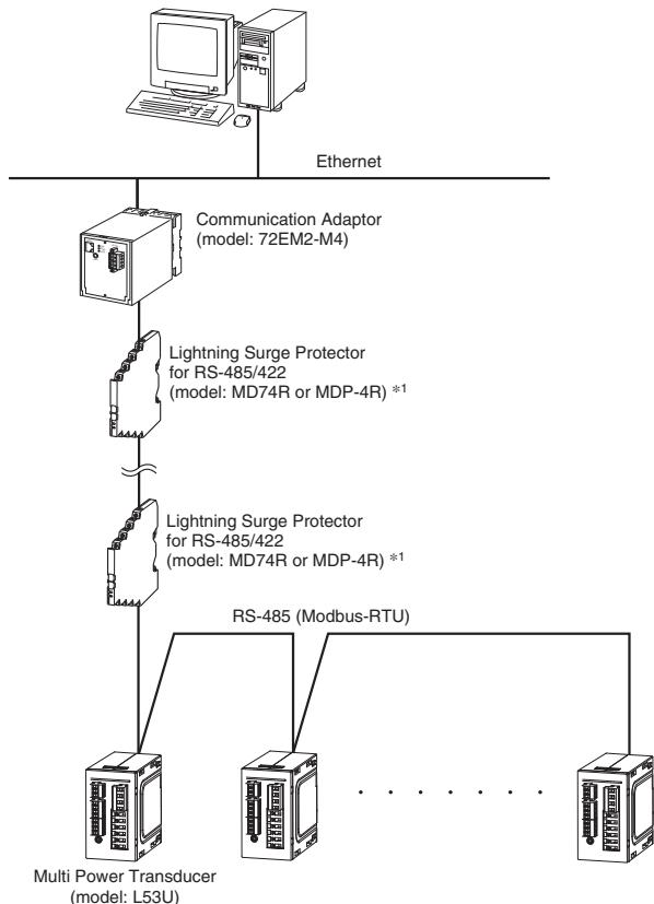
\*1. Insert lightning surge protectors recommended in this example if necessary.
