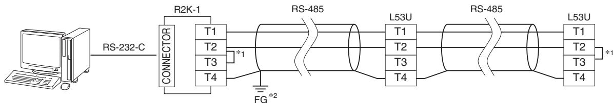
\*1. Internal terminating resistor is used when the device is at the end of a transmission line.
