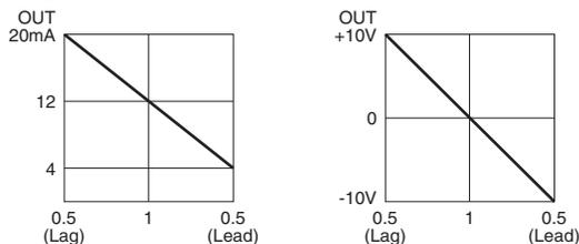
Note: When there is 5% or less of the rated input current, the transducer output equals approximately to '1'.
