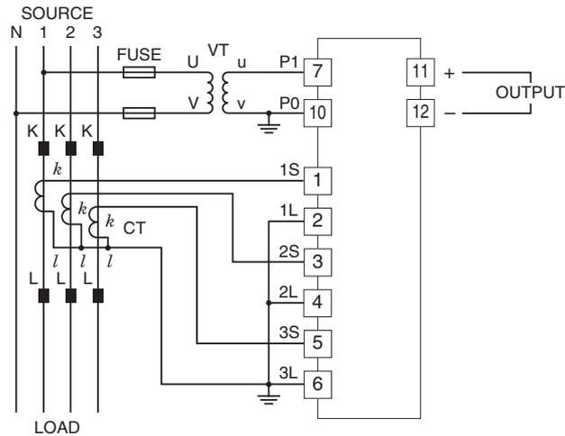
**EXTERNAL DIMENSIONS & TERMINAL ASSIGNMENTS unit: mm [inch]**
