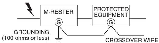
A crossover wire between M-RESTER ground and ground or metallic housing of equipment is required for protection.
