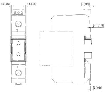
The Single Mount Adaptor cannot be combined with the Wiring Bridge (model: CNB).
