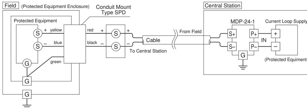
Connect the Conduit Mount Type SPD's green leadwire to the ground terminal inside the protected equipment enclosure to ground through the enclosure's outside ground terminal.
