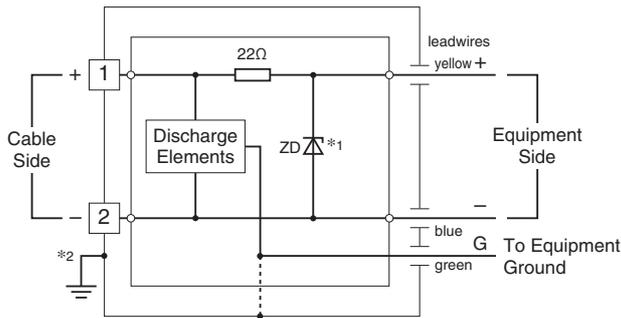
\*1. The zenor diode has polarity. Zero-cross signal cannot be connected.
