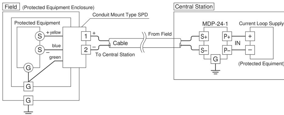
Connect the MD6T's green leadwire to the ground terminal inside the protected equipment enclosure to ground through the enclosure's outside ground terminal.
