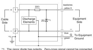
\*1. The zenor diode has polarity. Zero-cross signal cannot be connected.\*2. Use only when the signal line require functional grounding. This is NOT for surge protection.
