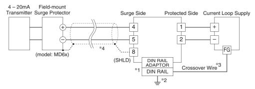
\*1.Oxide film on the surface of an aluminium rail may lower the electric conductivity between this module and the ground. Use a steel or copper rail.
