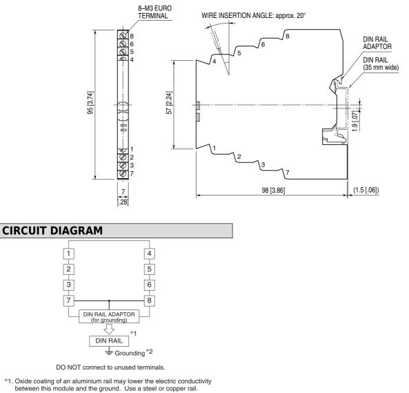
\*2. Be sure to ground the DIN rail. Recommended grounding resistance ≤100Ω
