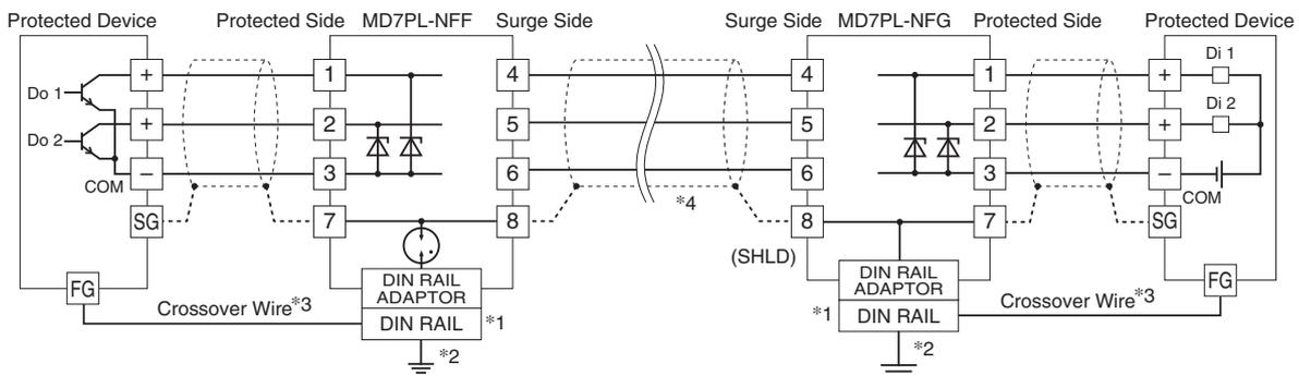
\*1. Oxide film on the surface of an aluminium rail may lower the electric conductivity between this module and the ground.
