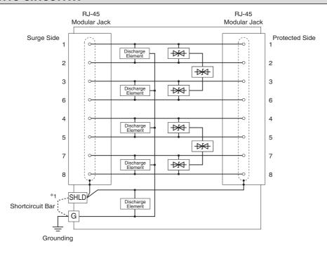
\*1. Remove the shortcircuit bar when the LAN cable's shield wire is floating. Note: Line to line (PoE): Terminal 1 & 2 to 3 & 6, 4 & 5 to 7 & 8
