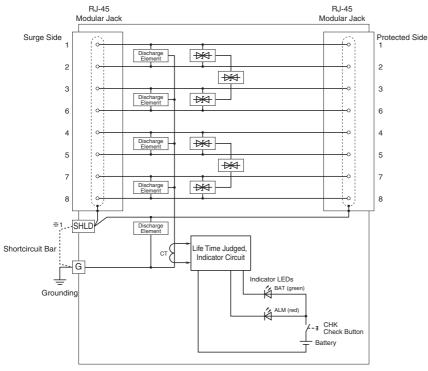
\*1. Remove the shortcircuit bar when the LAN cable's shield wire is floating. Note: Line to line (PoE): Terminal 1 & 2 to 3 & 6, 4 & 5 to 7 & 8 Line to line (pair): Terminal 1 to 2, 3 to 6, 4 to 5 and 7 to 8
