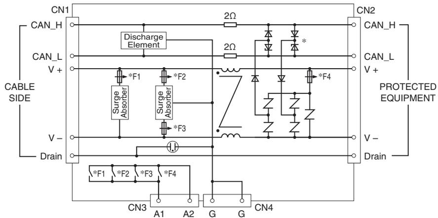
\*DO NOT CONNECT the communication line across CAN\_H and CAN\_L.
