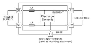
Note: When the head element is removed, the line will be open.
