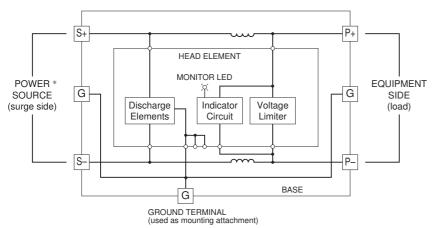
$<sup>^{*}</sup>$  Use a DC power source with the overload current protection function. (maximum output current 1A)
